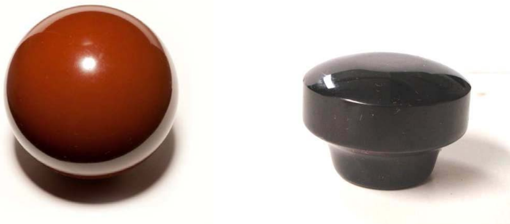
Fig. 1.1. and 1.2.: Bakelite billiard ball on the left and gear shift, artifact collection, NMAH, Smithsonian Institution (image credit photo on the left: Donald Hurlbert, Smithsonian) Whereas the need for a substitute for ivory for manufacturing billiard balls would have inspired John W. Hyatt, the inventor of celluloid, Baekeland was more interested in applications for automobiles, among other technical uses.
